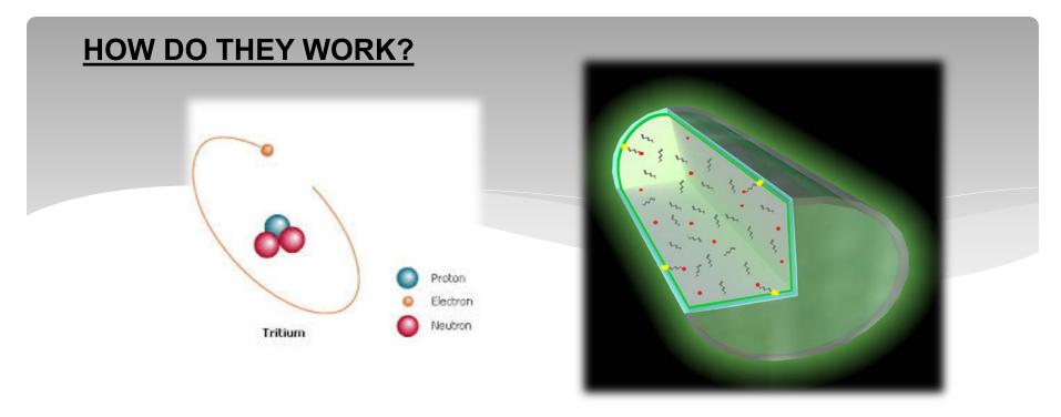
A tritium light source takes advantage of the radioactive properties of tritium gas (a special type of hydrogen gas) to cause the internally coated surface of a light source to glow.
